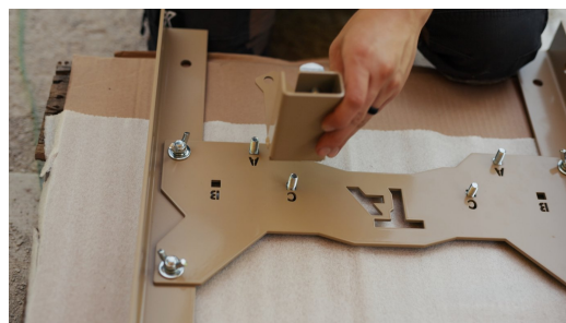
Installing a leg bracket onto the base center
