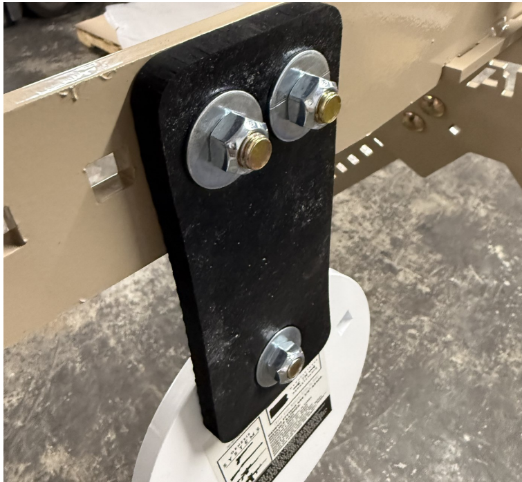
Correctly torqued strap bolt: the washer presses lightly into the rubber with a slight bulge. No more.
