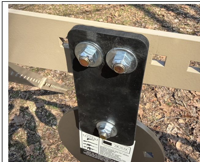
Single splice layer: standard 1/2" x 1.5" carriage bolt.
